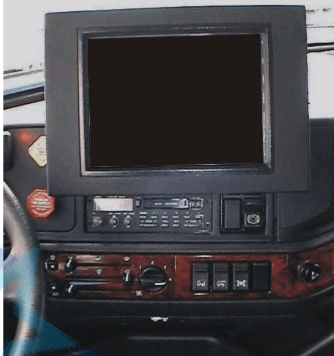
Figure 3.8 Placement of the display inside the experimental vehicle
